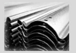
**CURTAIN (LATH)**: Constructed from 75mm wide curved interlocking galvanised steel 22swg solid, complete with cast end locks
